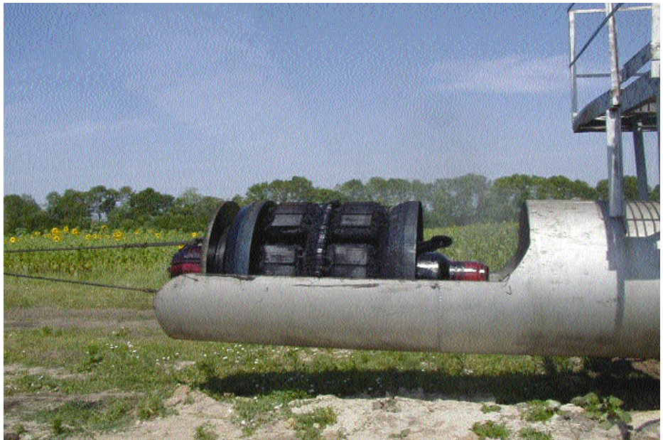
Figure 4.46 48 inch dual diameter single section MFL inspection tool with active speed control at receiver
