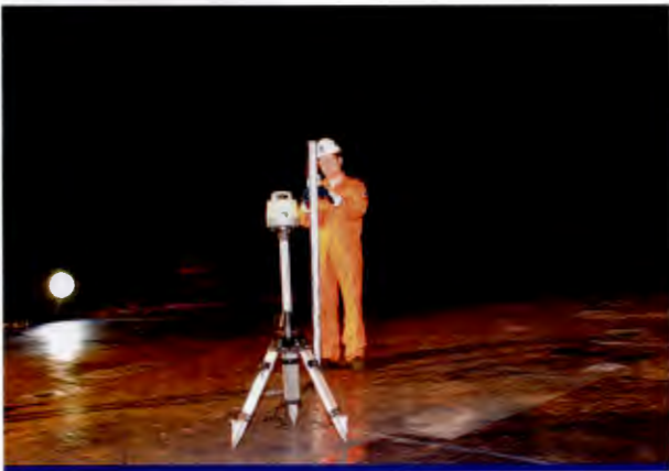
Figure 3. A gyroscopic balanced laser head is used to perform laser profiling services.
