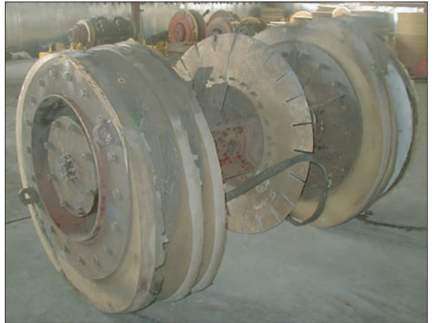
Fig. 2. Cleaning tool after a 50-km run through black powder.
