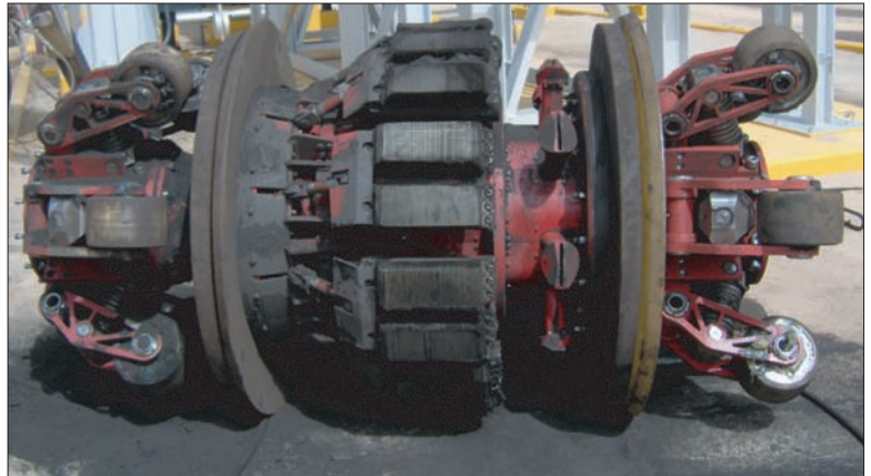
Fig. 4. Cleaning tool after more than 170 km in a gas line containing dry black powder.
