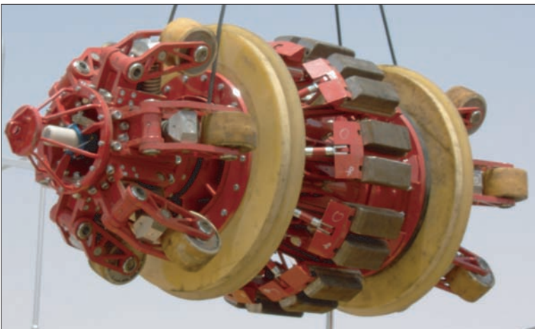
Fig. 1. Rosen 48-in Black Powder Cleaning Tool before launching.
