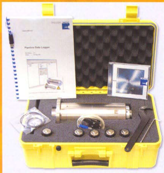
Figure 2. Pipeline data logger in carrying case.
