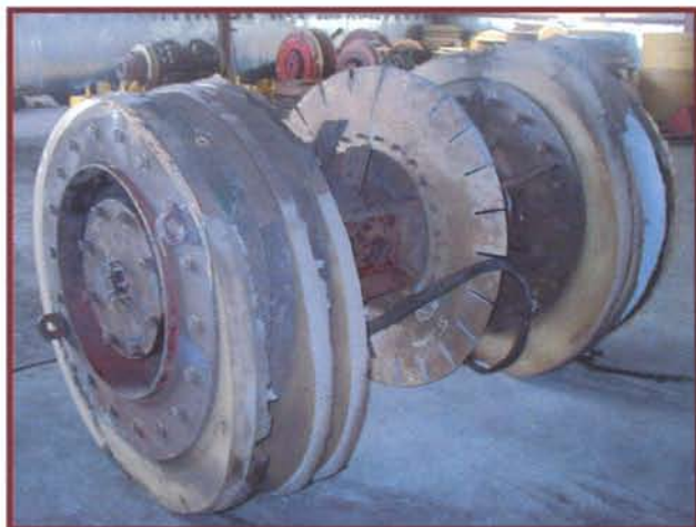
Figure 2. Cleaning tool after a 50 km run through black powder.
