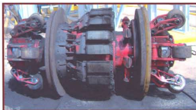
Figure 4. Cleaning tool after more than 170 km in a gas line containing dry black powder.
