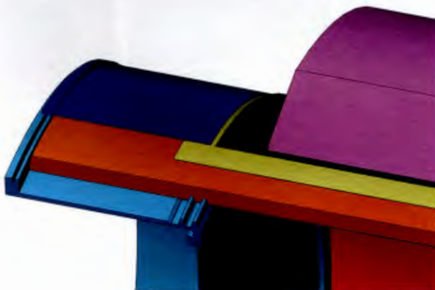
Figure 4. Outer cap with inner cap zip-lock system.
