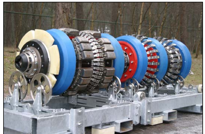
Figure 2: ILI multipurpose 24” tool. Combining MFL technology with high quality geometry inspection. Two measurement planes for the geometry sensor are required to provide full coverage under all operational conditions.
