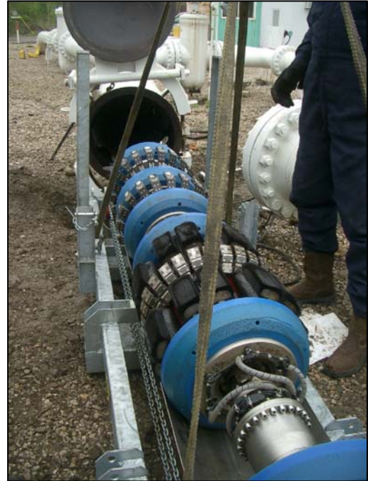
Figure 7: Multipurpose toolMFL, HighRes Geometry and IMU, at the receiver site.
