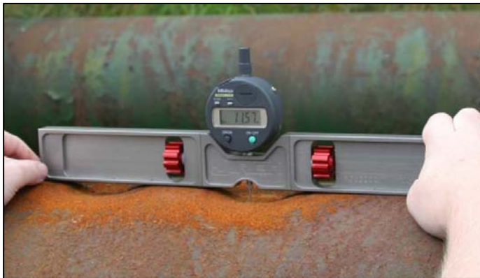
Figure 9: Artificial dent with almost rectangular contour. Inspection data obtained with the 16" ILI system (below). The characteristic shape is well reflected within the data.
