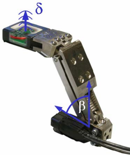
Figure 4: Combination of conventional mechanical caliper concept(B) with a touchless operating proximity sensor (d).
