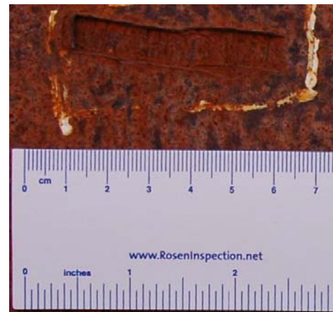
FIGURE 13: PHOTOGRAPH OF GOUGE USED IN CURRENT PULL TESTS.
