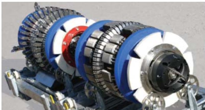
Figure 1: Combination of inspection technologies on a single 30" ILI tool. The front unit consist of a high-resolution MFL unit, the second unit is utilizing a combination of high-resolution geometry sensor with SIC probes.
