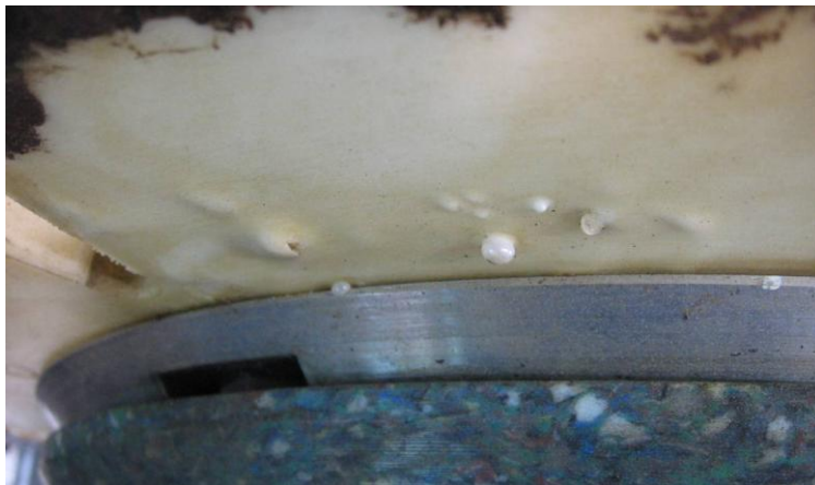
Figure 7: Guiding disc of 24" MFL in the workshop with visible bubbles.
