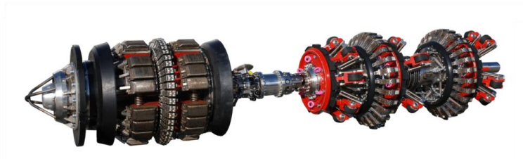
Figure 9: Combined in-line inspection with MFL technology (front), high-resolution geometry assessment (rear), and eddy current sensors for the detection and characterization of shallow internal corrosion (rear).
