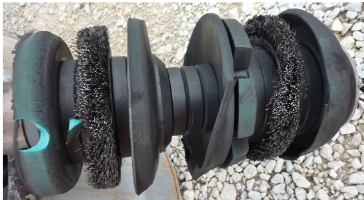
Figure 2: Ammonia PUR on a 6" pull unit after 82 km and 60 hours exposition time.
