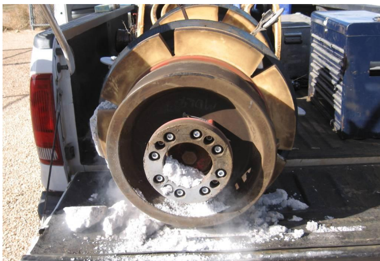
Figure 3: Geometry tool after 116 km in high pressure CO 2 .
