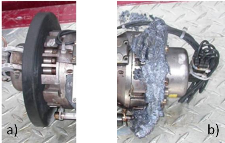
Figure 1: Polyurethane cup samples exposed to Ammonia over a period of 24h. a) Optimized composition b) Standard polyurethane
