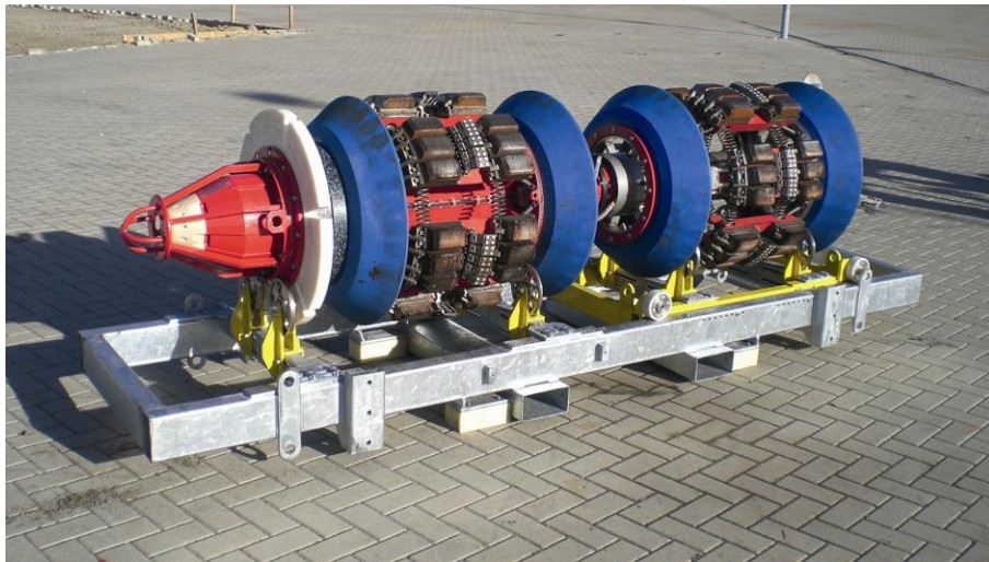
Figure 1: ROSEN's 26"/30" multi-diameter MFL tool with speed control
