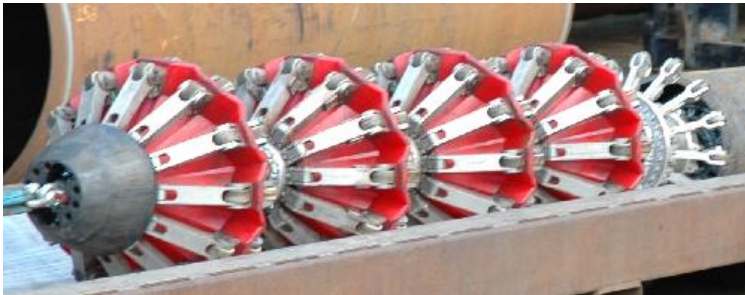
Picture 6: Multi-diameter sealing unit
