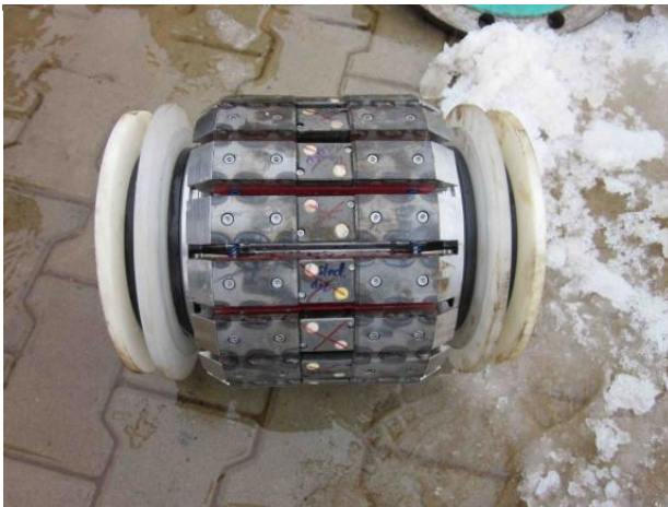
Picture 11: 10" MFL metal loss BiDi tool
