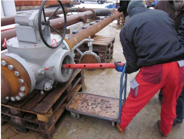
Picture 10: Ball valve with cleaning tool launcher / receiver
